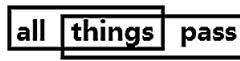
Fig. 1 N-gram language model. For N = 2 , the model treats the English sentence “ all things pass ” as being constructed from the bi-grams ( all, things ) and ( things, pass ).
