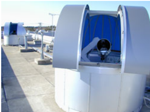
[Fig. 3] Stationary satellite optical observation system The two (2) telescopes, front and back, are alternately operated and maintained.
