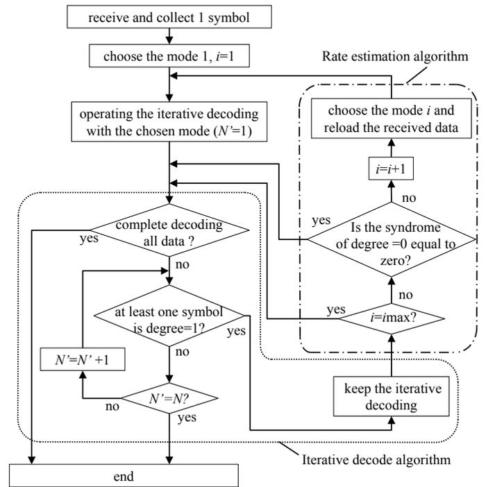
Fig. 4 Proposed algorithm of iterative decoding with rate-estimation.
