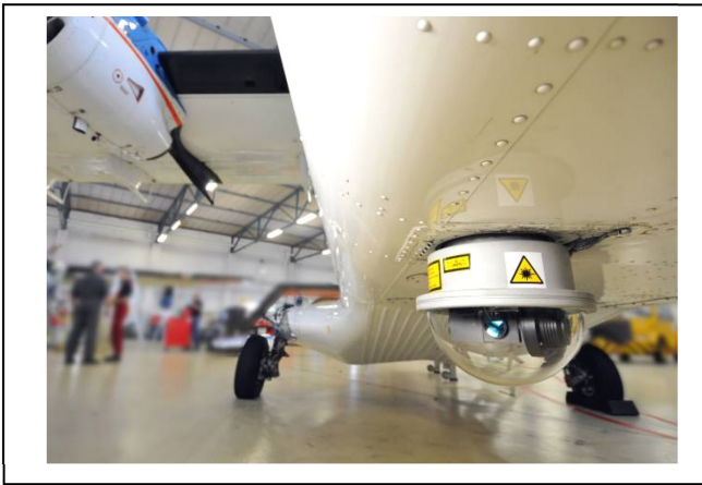
Figure 2. Aeronautical downlink terminal, attached to the fuselage of DLR's DO-228 aircraft
