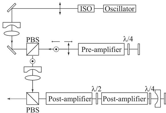
Fig. 3. Schematics of the laser system.
