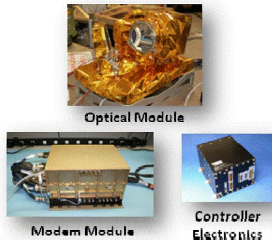
Figure 1. The Lunar Lasercom Space Terminal (LLST)
