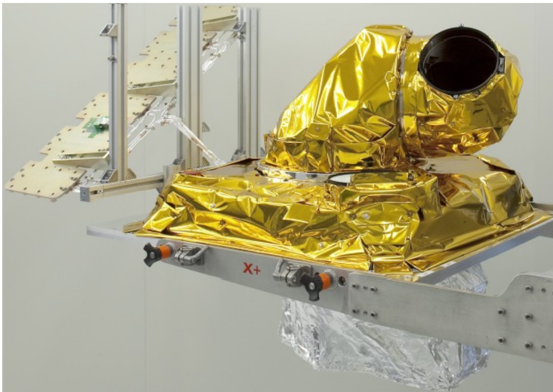
Figure 2. TESAT Laser Communication Terminal (LCT) baselined for European Data Relay System (EDRS) and Global Monitoring for Environment and Security (GMES). The photo displays the LCT which has been integrated on the Alphasat GEO spacecraft.
