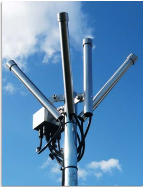
Figure 10. Cloud age and ceilometer instruments
