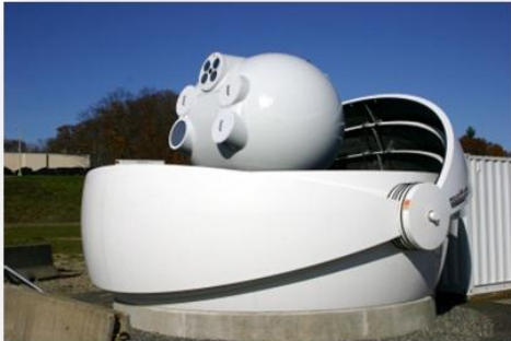
Figure 5. The Lunar Laser Communication Demonstration's (LLCD) Transportable Lunar Lasercom Ground Terminal
