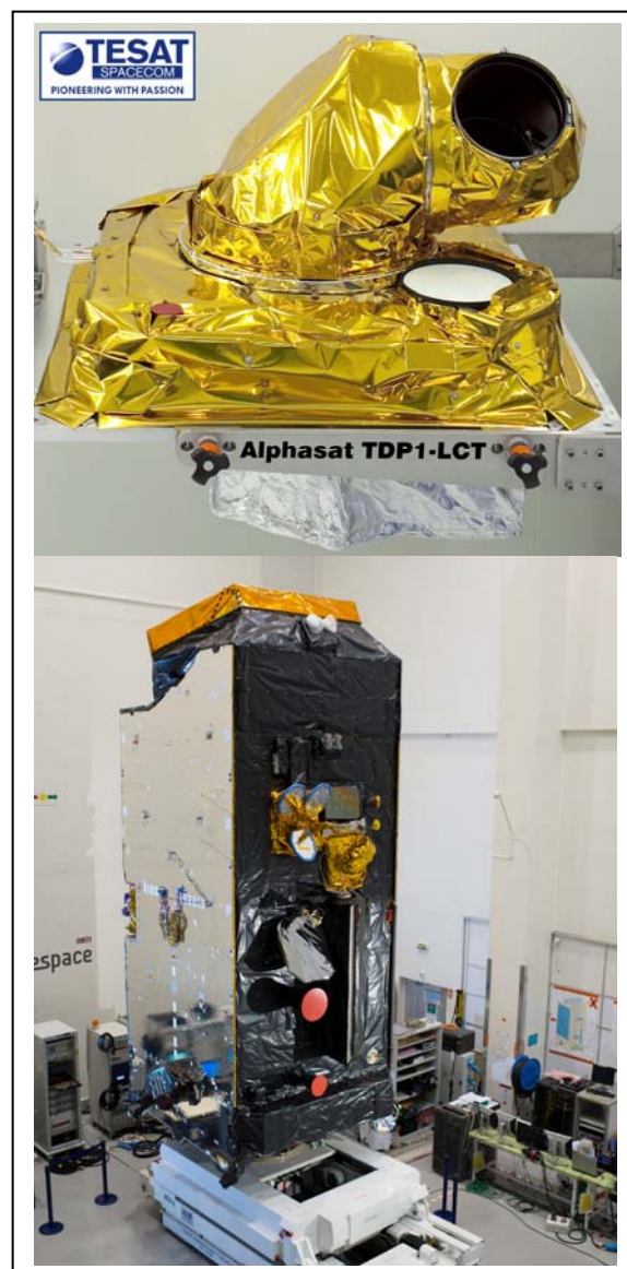
Fig. 7. Top: Alphasat LCT before delivery to space craft. (Picture courtesy TESAT) Bottom: LCT embarked on Alphasat as TDP1 (picture courtesy ESA).
