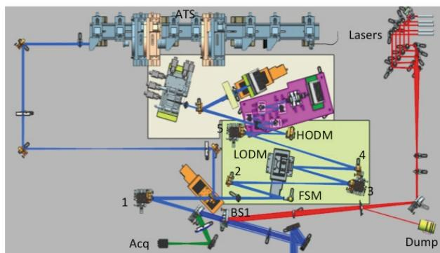
Figure 2: The IOS opto-mechanical layout. The Transmit arm is marked in red the Acquisition arm in green and the AO arm in blue. The WFS is mounted on the purple breadboard. The remaining components in the AO arm are divided between the
