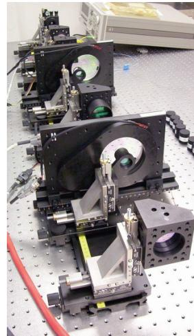
Figure 3. The LOGS atmospheric turbulence simulator built into the IOS optical train allows the simulation of a variety of atmospheric conditions.
