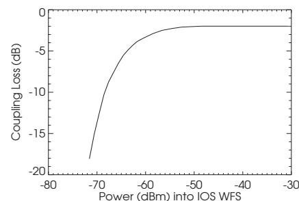
Figure 4: Fiber coupling loss as a function of the downlink power entering the IOS wave front sensor.
