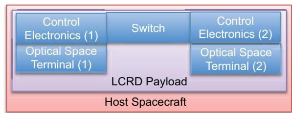
Figure 1. LCRD payload to be on commercial communications satellite
