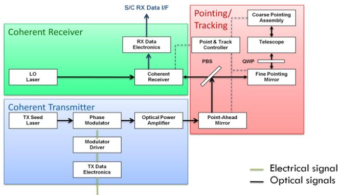
Fig. 1. LCT block diagram.
