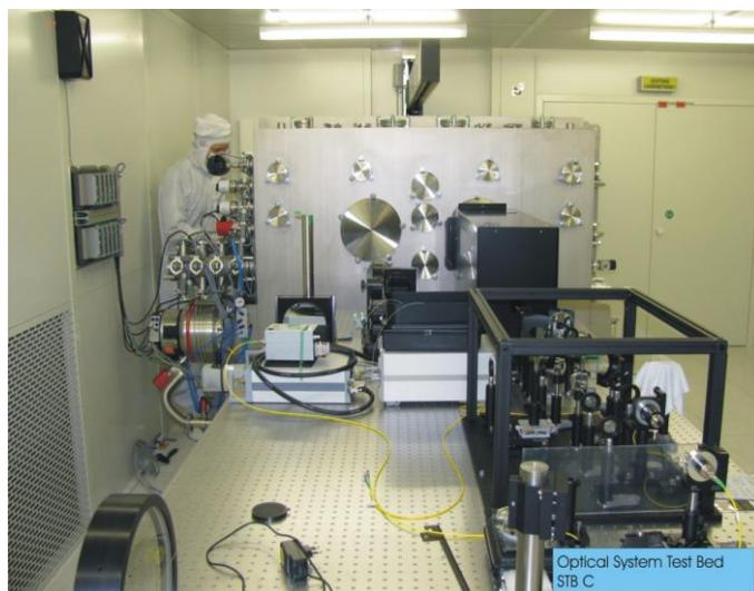
Fig. 5. Class 100 (ISO 5) cleanroom- showing thermo vacuum chamber (background) for the LCT and wafe front and communication analization equipment located in the front.
