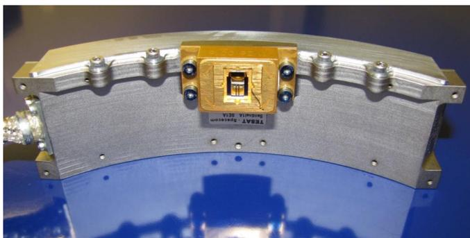
Fig. 4. Optical Encoder
