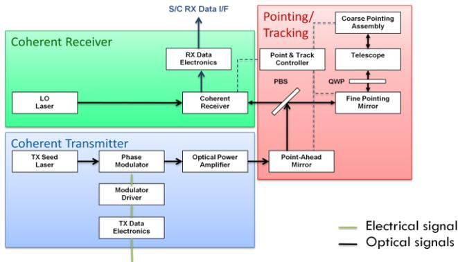
Fig. 1. LCT block diagram.
