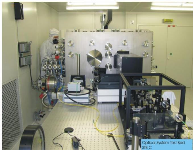
Fig. 5. Class 100 (ISO 5) cleanroom- showing thermo vacuum chamber (background) for the LCT and wave front and communication analization equipment located in the front.
