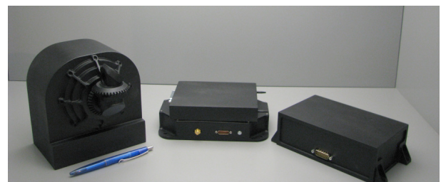
Fig. 2. OPTEL- \mu space terminal, 3 main units, rapid prototyping models (from left: Optical Head, Laser Unit, Electronics Unit)
