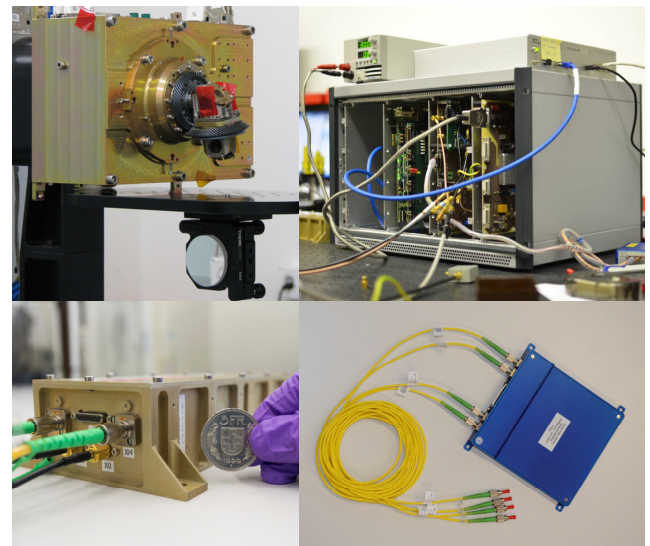
Fig. 14. The Space Terminal (DUT1) consists of 4 boxes (clockwise from upper left: Optical Head Unit, Electronics Unit, Optical Fiber Amplifier, Pulse Laser Transmitter)
