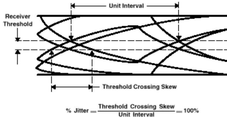
**Figure 14. Measuring Signal Transmission Quality**
