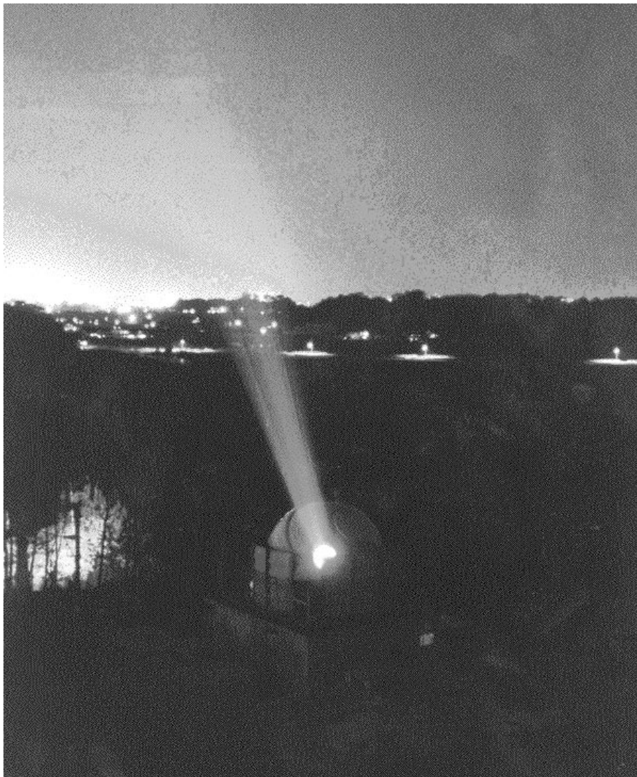
Photo. KSP SLR system under test observation at Kashima. During period of January 30-February 14 in 1997, Kashima and Koganei stations have made observation for major geodetic satellites LAGEOS, AJISAI, STELLA and Starlette in order to check out ranging precision and accuracy stability. Forty five LAGEOS1&2 passes in total were analyzed to produce baseline length between Kashima and Koganei with accuracy of 20-30 mm, although the system were not fully equipped with those to meet final specification. The four systems have get together and will be configured with a single telescope for colocation, a comparison observation with each other at Kashima. (Hiroo Kunimori)
