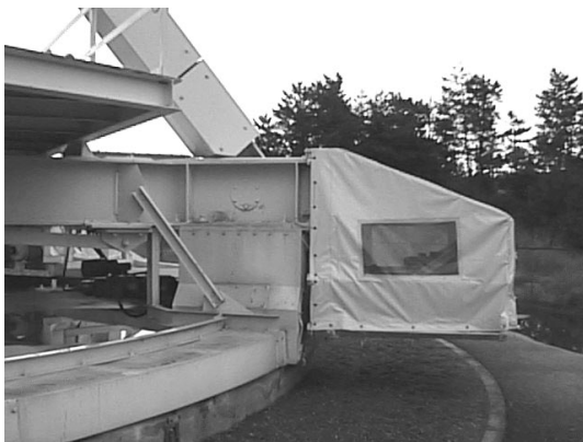
Figure 1. An AZ motor cover to protect the motor.
