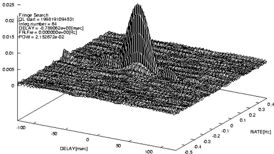
Figure 4. Detected fringe from the observation towards NRAO530. The integration time is 64 seconds (July 10, 09:45:31-09:46:35 UT). The X-band IF signal from the Key Stone Network antenna (8100-8600MHz) was converted to the baseband (0-500MHz). And a bandpass filter (bandwidth : 25 MHz, center frequency : 212 MHz) was used before the baseband signal was sampled by the TDS784 sampler unit.
