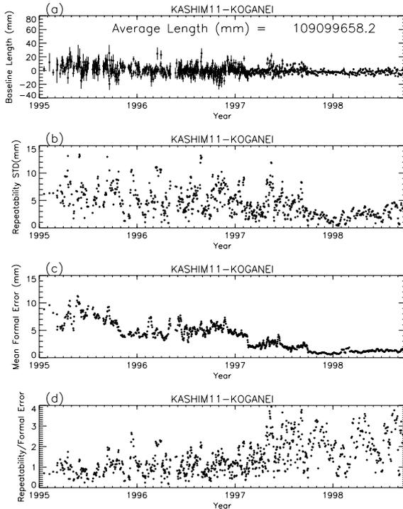
Figure 2. Evolution of baseline length between Kashima and Koganei (a), repeatabilities (b), mean formal errors (c), and ratio of repeatability to mean formal error (d) of five consecutive samples of baseline length.
