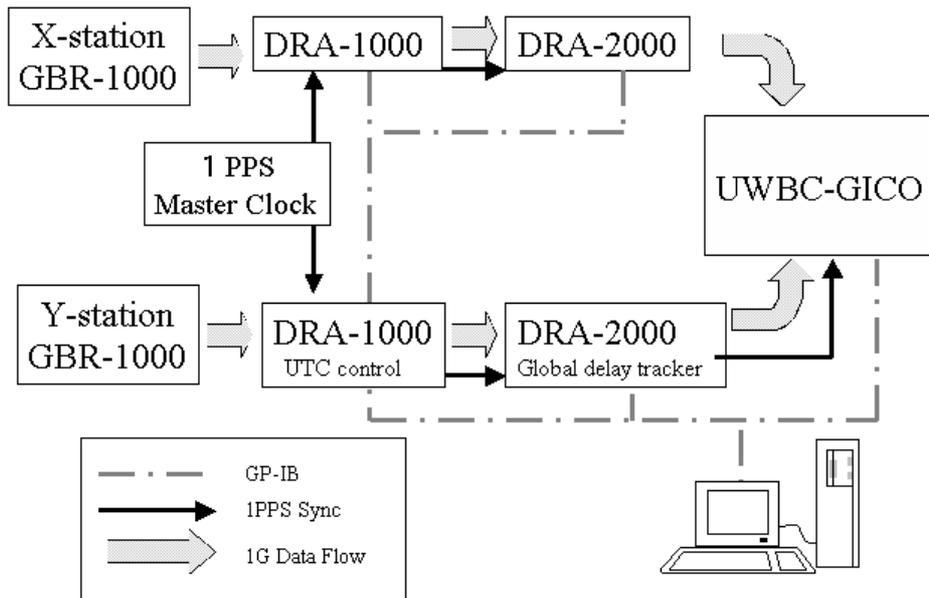
Figure 2. Schematic diagram of the system configuration for correlation processing.
