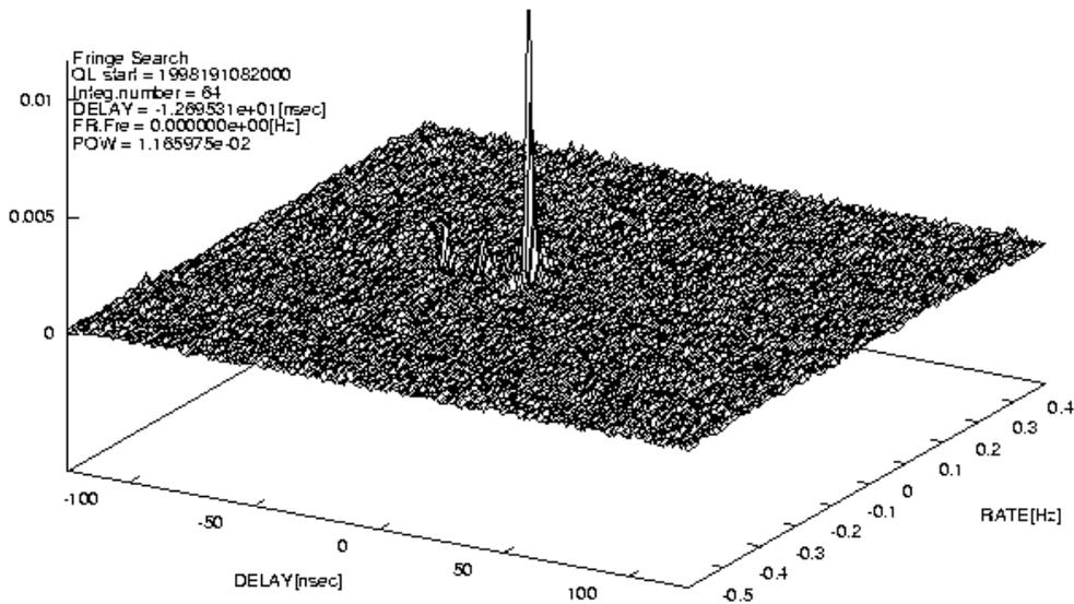
Figure 3. Detected fringe from the observation towards 3C345. The integration time is 64 seconds (July 10, 08:20:00-08:21:04 UT). The X-band IF signal from the Key Stone Network antenna (8100-8600MHz) was converted to the baseband (0-500MHz) and sampled by the TDS784 sampler unit.
