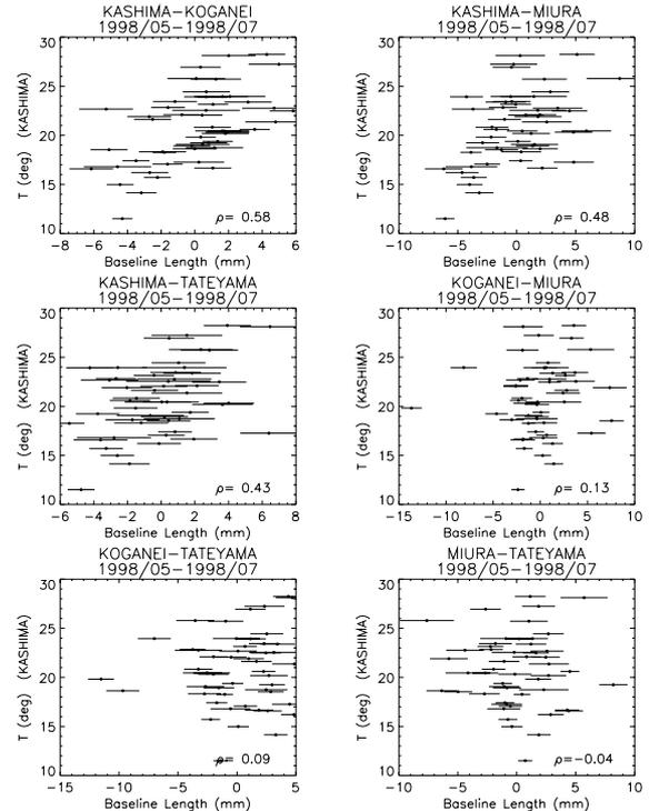
Figure 3. Scatter plots of temperature and the fluctuation of baseline lengths for the period May 1998 to July 1998.
