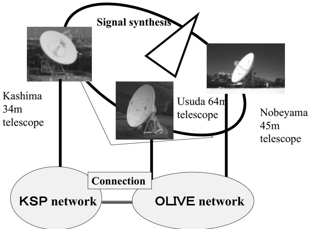
Figure 1. Outline of virtual telescope using high speed communication
