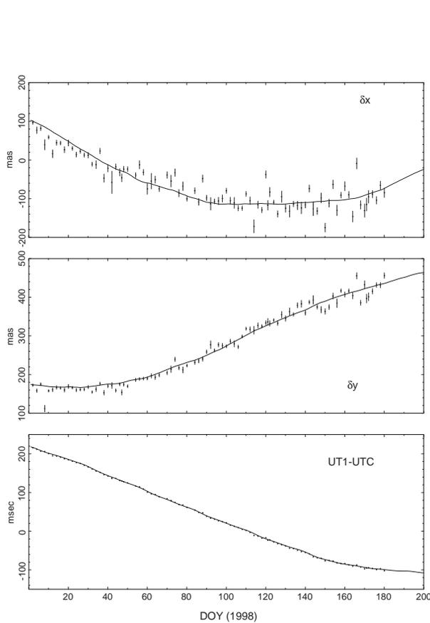
Figure 2. Estimated earth's rotation pole position ( $\delta x$  and  $\delta y$ ) and UT1-UTC from the KSP VLBI data. Solid lines are indicating EOP97C04 values provided by IERS.
