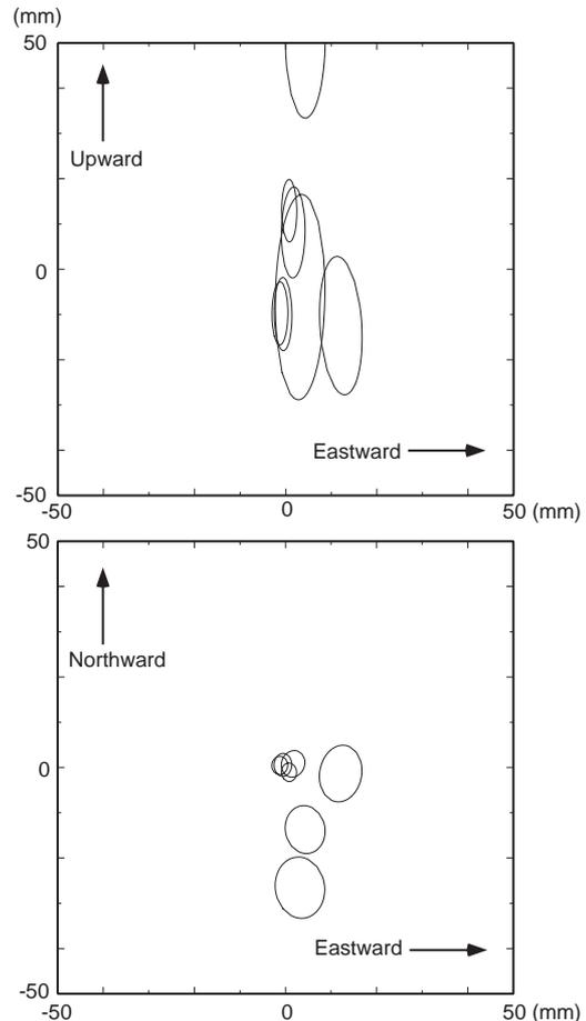
Figure 1. Estimated site position of the KSP Kashima VLBI station. Error ellipses are  $1\sigma$  formal errors.
