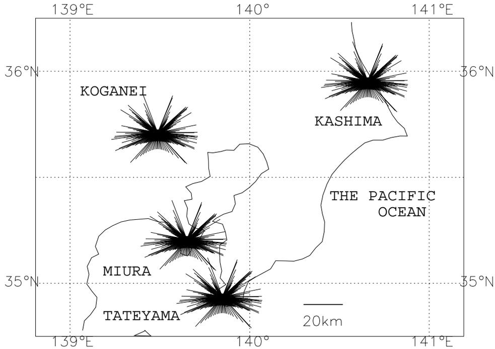
Figure 4. Ray paths projected on the earth surface during a VLBI session at each KSP station. The ray paths plotted have altitudes less than 4 km.
