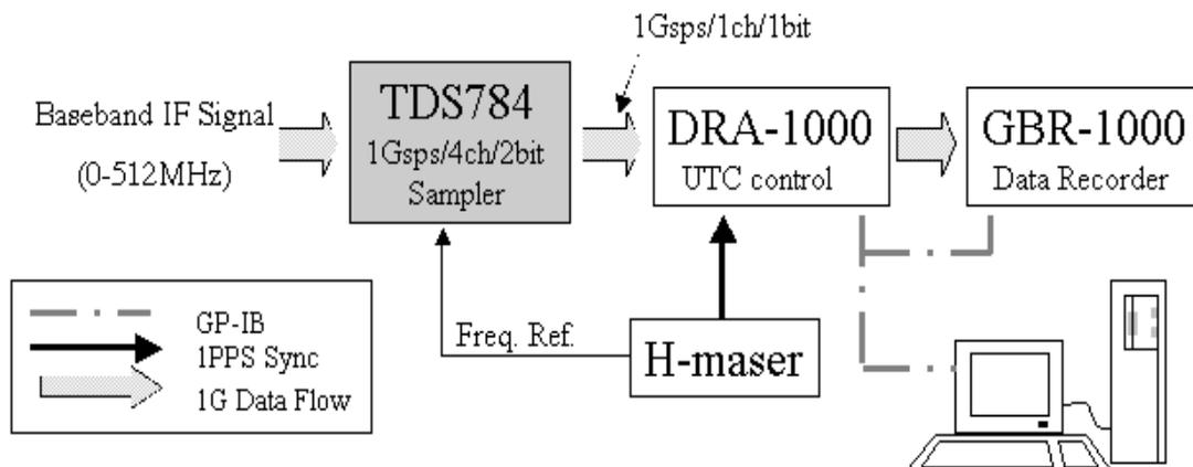
Figure 1. Schematic diagram of the system configuration for observations.
