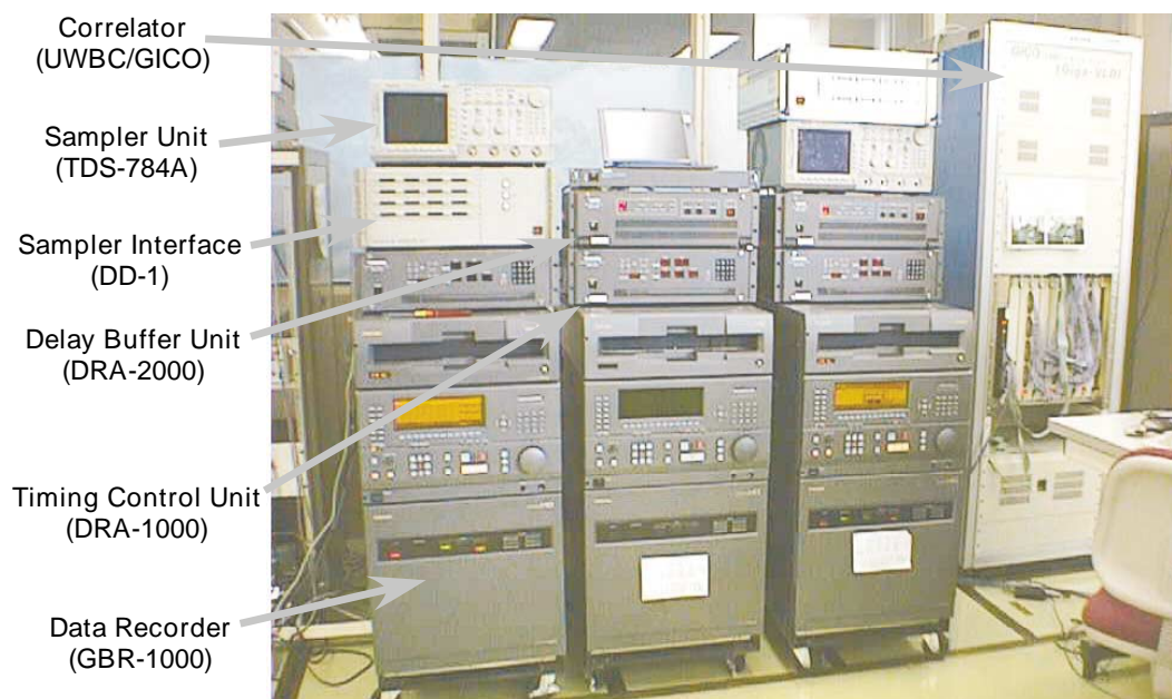
Figure 1. A picture of the whole system of the giga-bit VLBI system.
