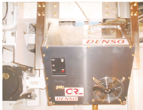
Figure 5. HTS filter subsystem installed at LNA output.
