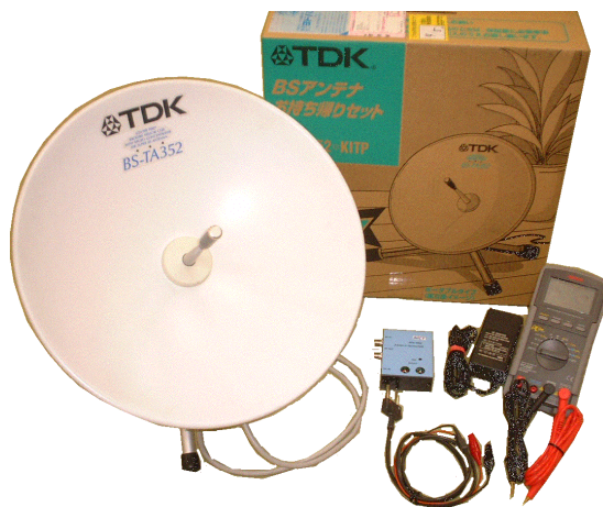
Figure 1. CARAVAN-35 package is being distributed from EDC. 35- cm dish, RFD-1500 backend and DVM are the key components. By using RS-232 / USB readout of DVM, students can experience pen-recorder type basic observation essential in radio-astronomy.
