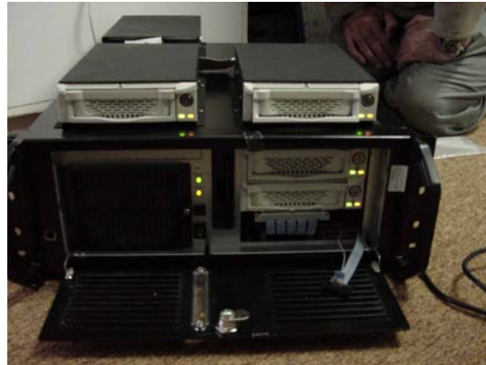
Figure 3. The VLBI system with 4 demountable 200GB IDE drives.
