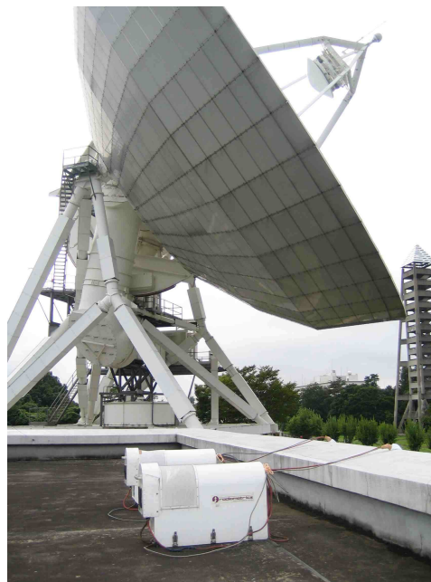
Figure 1: WVR (Radiometrics TM WVR-1100) measurements at Tsukuba. The Tsukuba 32-m antenna of GSI is shown behind the WVRs.
