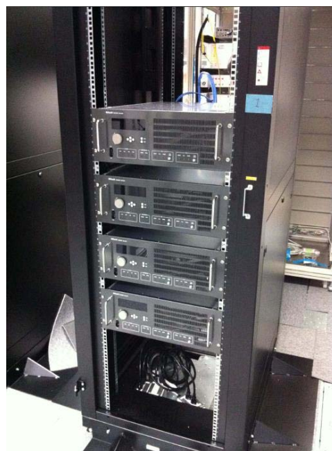
Figure 1. K6/iDAS sampler units in rack.
