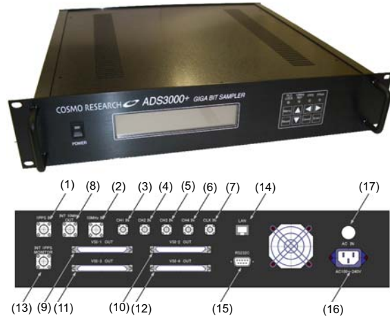
Figure 2. Outlook picture (top) and backside view (bottom) of the ADS3000+ are displayed. External reference input of 10MHz(2), 1PPS(1), and internal 10MHz(8) and 1PPS(13) are interfaced with BNC. RF signal inputs (3,4,5,6) are connected by SMA. Each of VSI-H output interface (9,10,11,12) supports data rate up to 2048 Mbps (64 MHz clock via 32 wires).
