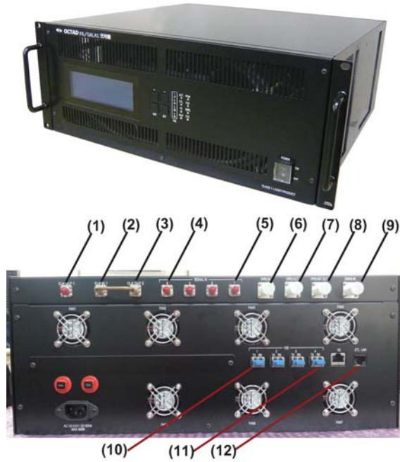
Figure 3. Upper figure shows outlook of direct sampler K6/GALAS. Radio frequency analog signal is converted to digital signal by 16,384 MHz sampling 3 bit quantization. Specified four 1-GHz bandwidth signals ( 2048\text{Mps} \times 1\text{bit} \times 4\text{ bands} ) are extracted via digital baseband conversion function. The data is output in the stream of VIDF/UDP packets from 10GBASE-SR interfaces. Lower figure shows back-side view of the sampler. Sampling clock is selection by connecting one of clock outputs at (1) and (3) to clock input (2). 3.5mm connectors (4)-(5) are RF signal inputs. External reference 10MHz signal and 1PPS are input from (9) and (6), respectively. Returning 1PPS (7) and internal 1PPS (8) are also available. Four 10GBASE-SR interfaces (10)-(11) are for data output and 100Base-T Ether connector (12) is used for external control.
