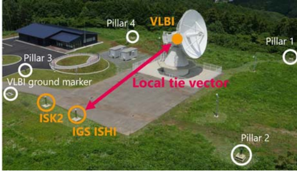
Figure 1. Panoramic view of the Ishioka station. Four pillars and a VLBI ground marker are arranged around the VLBI antenna and GNSS stations.
