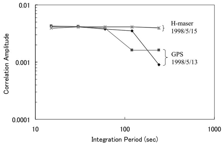
Figure 9. Relation between correlation amplitude and integration period for two test observations: in one H-maser clocks were used at both stations, and in the other a GPS reference receiver was used at one station.
