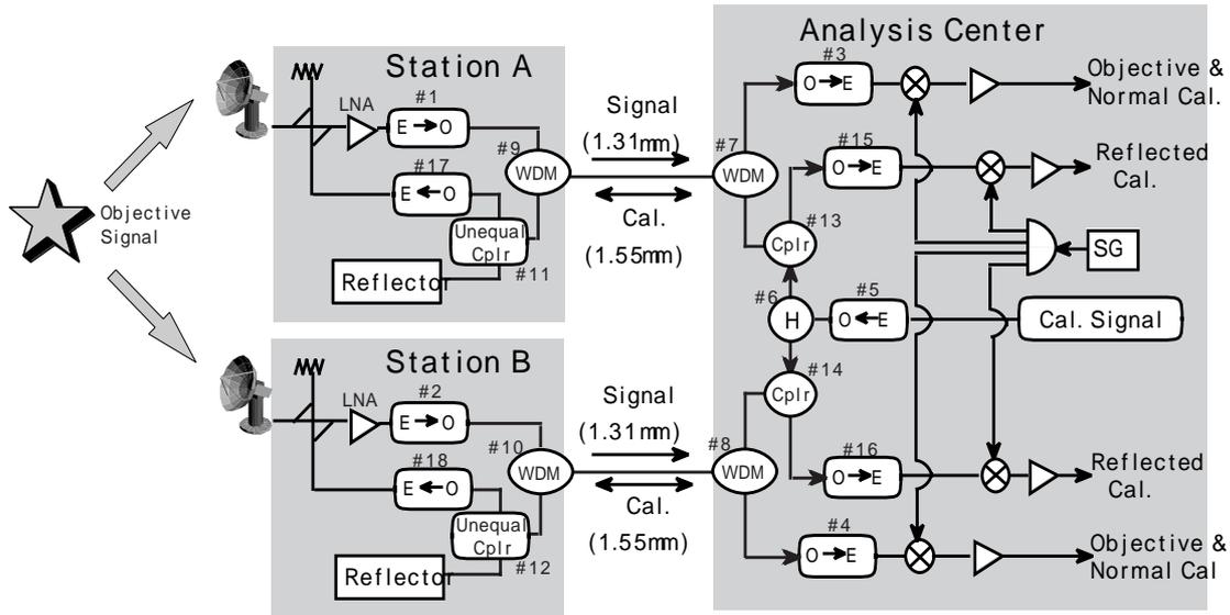
**Figure 6.** System configuration of the optical-linked RF interferometer.
