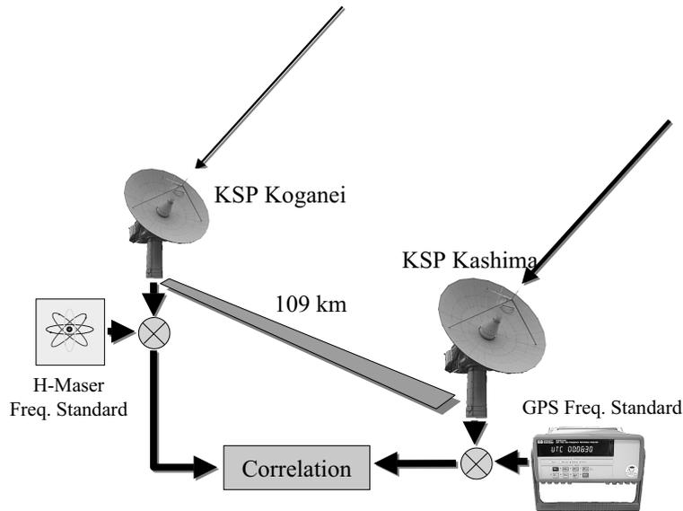
**Figure 7.** Configuration of test VLBI observation using GPS frequency standard.
