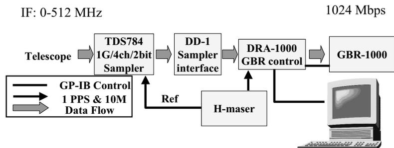
**Figure 5.** Schematic diagram of the Giga-bit VLBI system for observations.
