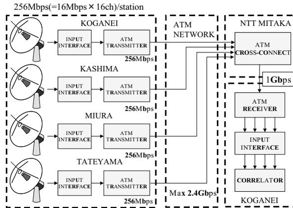
Figure 2. Block diagram of the KSP real-time VLBI system.
