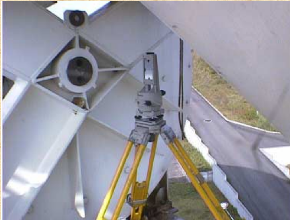
Ground survey target at VLBI reference point (Kashima)
