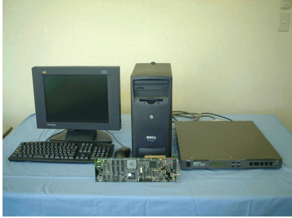
Fig. 3. PC-VSI system (left) and ADS1000 A/D sampler unit (right). The board in front of the PC-VSI system is the PC-VSI2000-DIM board.
