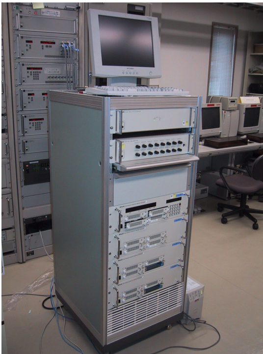
Fig. 1. The prototype K5 VLBI data acquisition system.
