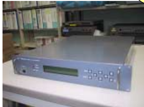
ADS2000 (64Msample/ch-sec, 16ch, 1bit or 2bits)
