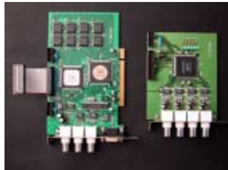
ADS2000 (64Msample/ch-sec, 16ch, 1bit or 2bits)
