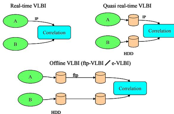
**Fig.4. Supposed Operational Mode of the Internet VLBI**
