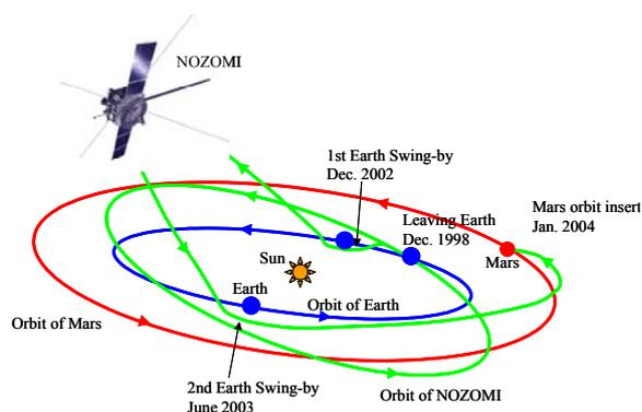
Fig.10. Trajectory of NOZOMI (after <http://www.isas.ac.jp/e/enterp/missions/nozomi/traject.html>)
