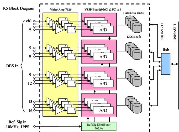
**Fig.2. A schematic block diagram of K5-VSSP system.**
