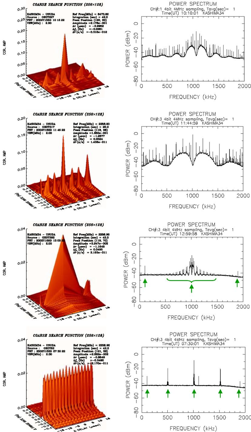
Fig.6. Fringes detected for GEOTAIL. Group delays can be determined without ambiguity excepting the lowest panel case.
