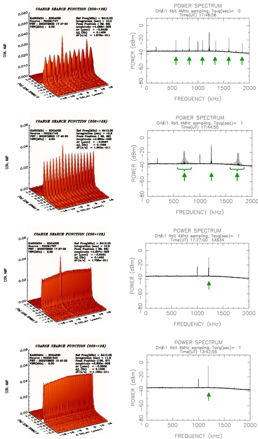
Fig.7. Fringes detected for NOZOMI. Group delays can be determined without ambiguity excepting the lowest panel case.
