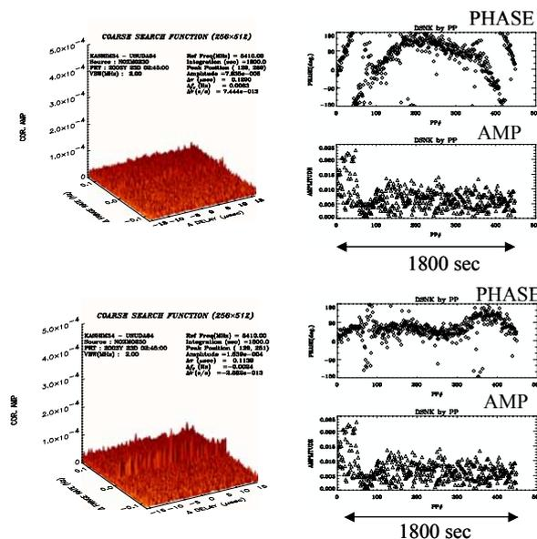
Fig.11. A normal fringe search for 30 minute scan data (upper two panels) and an improved fringe search (lower two panels).
