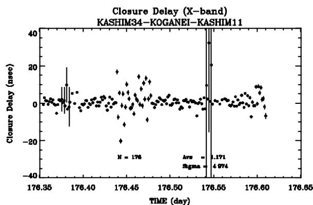
Fig.9 An example of closure delay test for GEOTAIL observations. Observations were carried out on June 25, 2002 at three stations, Kashima34, Kashima11, and Koganei11. Data with large error bars represent quasar observations. Although data are largely scattered around 176.45 days, standard deviation of total data is well less than 10 nsec.
