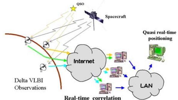
**Fig.1.** Concept of quasi real-time positioning of spacecraft using the Internet VLBI system.
