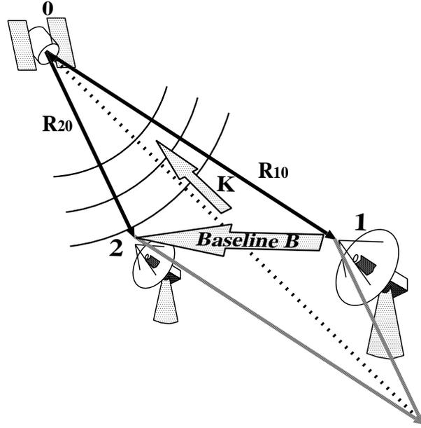
**Fig. 1.** Schematic diagram of pseudo source vector  $\mathbf{K}$ . The vector  $\mathbf{K}$  is on the diagonal line of the parallelogram composed from vector  $\mathbf{R}_{10}$  and  $\mathbf{R}_{20}$ .
