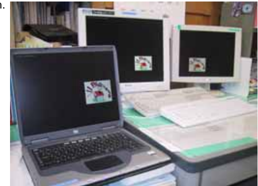
Figure 2:GRID VLBI correlator system consists of multiple PCs. In this picture, three standard PCs are correlating VLBI data using screensaver-type client programs like SETI@home.
