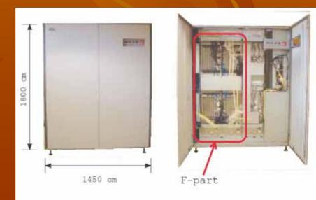
Figure 1: 4-Gsps 2-bit FX Correlator with 262144-point FFT
