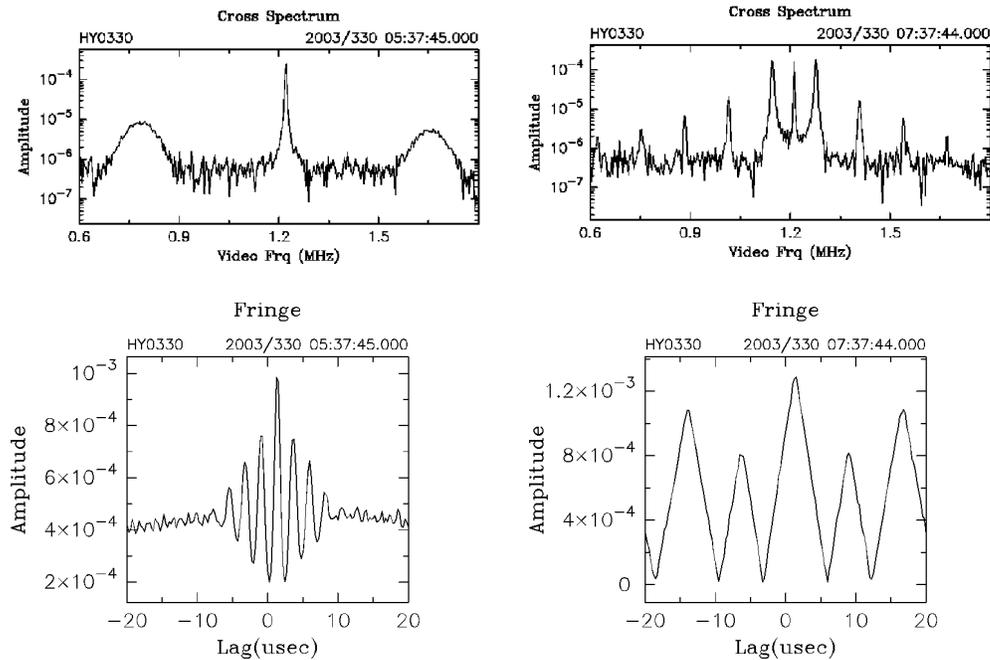
Figure 2: Frequency spectrum (upper panel) and delay resolution function (lower panel) of range signal (left) and telemetry signal (right), respectively.
