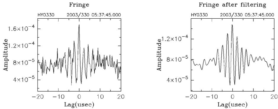
Figure 3: Effect of signal filtering. Signal to noise ratio of delay resolution function was improved by bandpass filtering of range signal (right) than before filtering (left).
