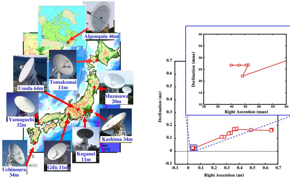
Figure 1: Celestial coordinates of NOZOMI estimated by VLBI observations on 4th June 2003 is plotted. The origin of plot is the orbit determined by R&RR measurements. Atmospheric delay was calibrated by means of GPS observations. Each points of plot are solutions with data sets as including from short baselines to long baselines. Magnified plot superimposed at the top is solutions including Algonquin related baselines.
