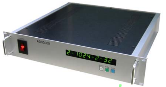
ADS3000 (2048Msample/sec 1ch 8bits + FPGA)
