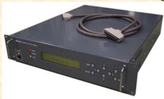
ADS2000 (64Msample/ch·sec, 16ch, 1 or 2bits)
