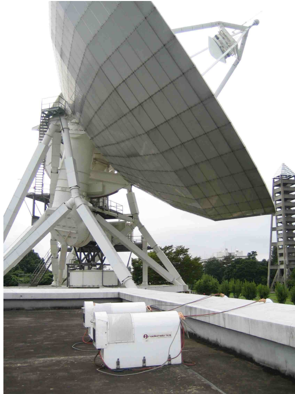
Figure 1. Two WVRs nearby Tsukuba 32 m station of GSI. Each WVR was equipped at Kashima and Tsukuba during the CONT05 campaign.
