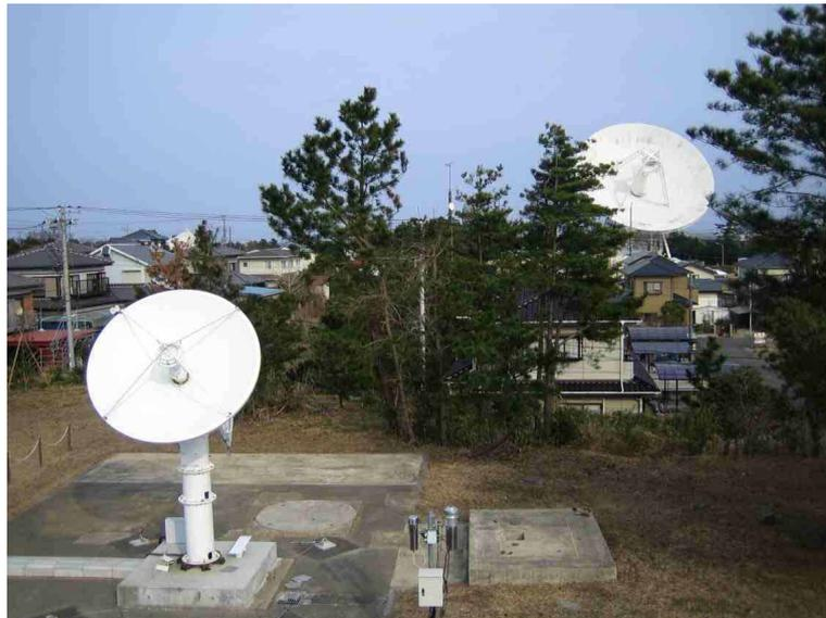
Figure 3. 2.4m antenna (front) and 34 m antenna (back) at Kashima during a fringe test.
