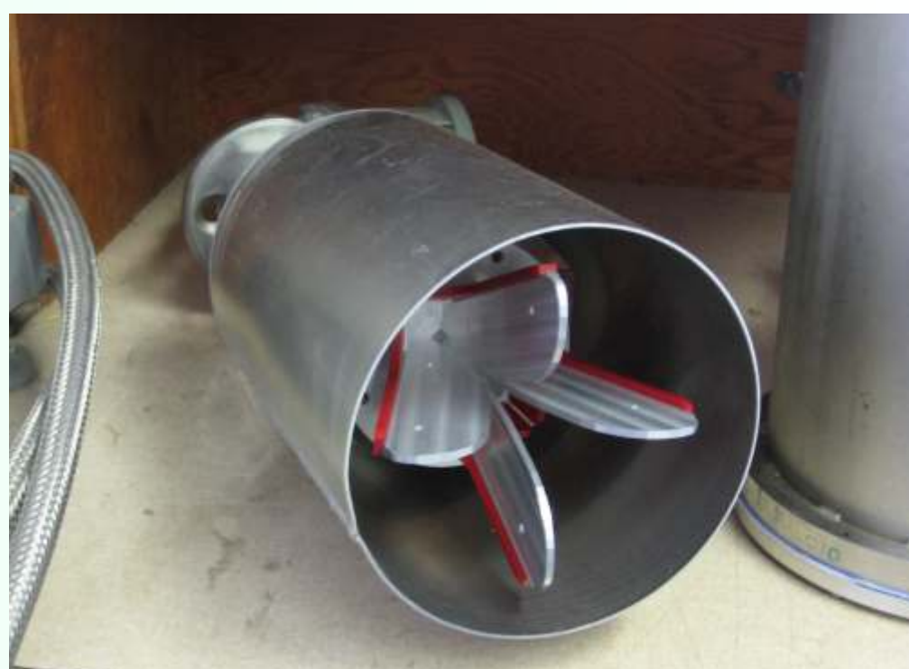
Figure 2. ETS-Lindgren quadridge broadband feed inside heat shield attached to the 15K station of the cryogenic refrigerator. Dewar is to the right.
