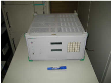
Figure 4. LD-pumped cesium gas-cell atomic frequency standard.
