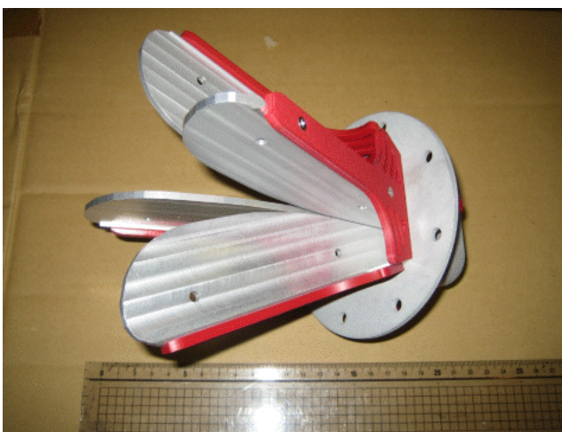
Fig.5. A quad-ridge horn antenna (QRHA). It can cover 2-18 GHz.
