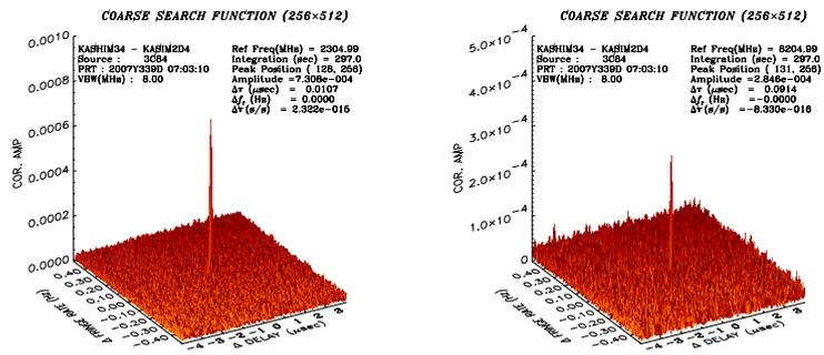
Figure 4. Fringes detected by CARAVAN2400 adopted by a QRHA. Left panel shows S band fringes and right for X band.
