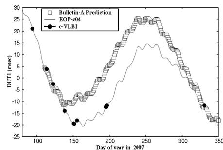
Figure 2. Comparison of UT1-UTC among EOPc04, prediction of Bulletin-A, and e-VLBI observation. Linear trend of UT1-UTC has been removed in advance. It is obvious that UT1 measured by e-VLBI observation has higher precision than prediction values.
