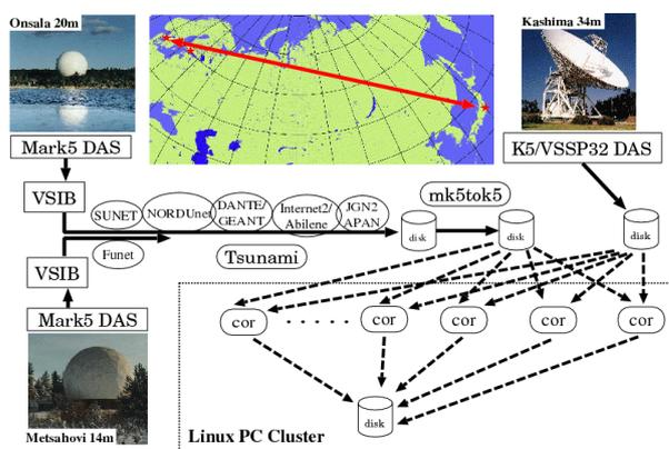
Figure 1. VLBI stations participating the Ultra-rapid UT1 measurements and a block diagram of data flow and data processing.
