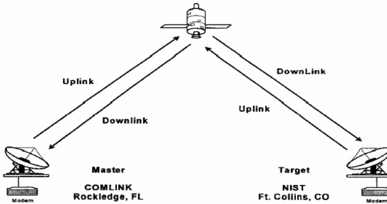
Figure 1. Basic Two-Way Satellite Time Transfer Link
