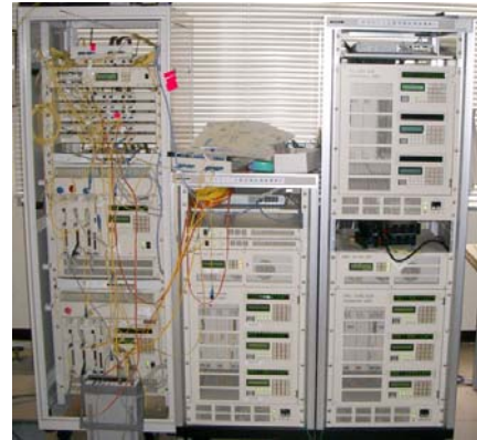
Figure 2: High speed hardware correlators with 2Gbps \times 6 baselines capability (center-right) and VLBI network adapter VOA-200 (left) developed by NAOJ.
