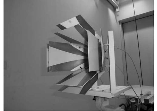
Figure 4. Experimental elements for wide-band feeds.
