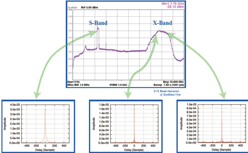
Figure 3. First fringe of DSAMS (Direct sampling applied for mixed signals) applied for geodetic VLBI. The sampling mode of ADX-831 is 2bit-1024Mps. Fringes of S-band and X-band were simultaneously obtained with the only one sampler.
