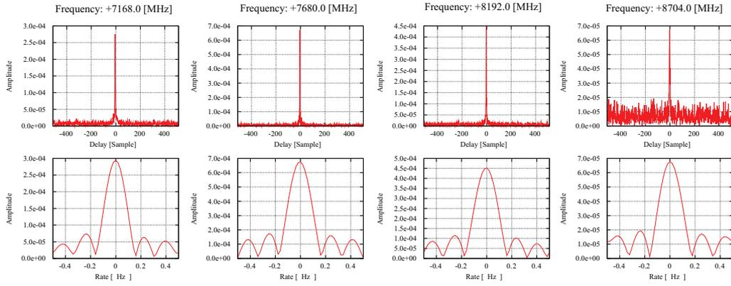
Figure 2. First fringe for DSAMS (Direct Sampling Applied for Mixed Signals) applied for X-band VLBI. The sampling mode of ADX-831 is 2bit-1024Mps. Each Fringes of four X-band were simultaneously obtained with “single” sampler.
