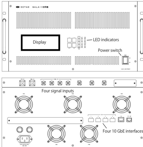
Fig. 1 The design of the direct sampler Galas.
