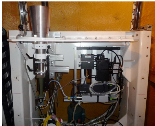
Figure 1. Prototype of Iguana Feed install at Kashima 34m antenna. SEFD is 1000 - 2000 Jy in 6-14 GHz frequency range.
