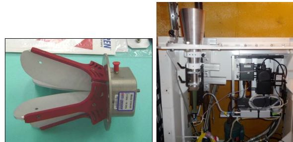
Figure 3, Quad Ridge Horn Antenna (Left) has 2-18GHz observation frequency range. This is used for 1.5-m and 1.6-m antenna. Right panel shows the new wideband feed, which has 6.4-15GHz frequency range, installed in the receiver room of Kashima 34m antenna.
