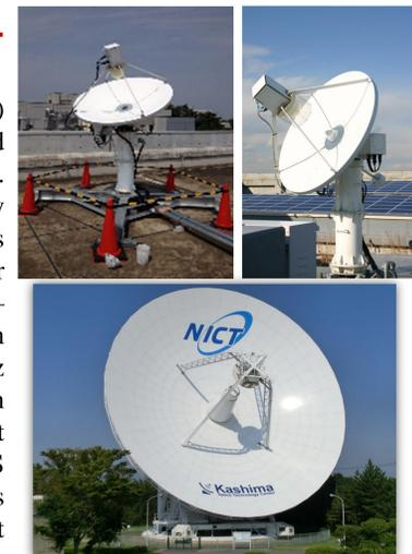
Fig. 4 Pictures of 3 radio telescopes of the GALA-V system. 1.6m antenna at NMIJ (top-left), 1.5m antenna at NICT/Koganei (top-right), and 34m radio telescope at NICT/Kashima(right).
