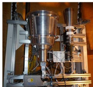
Fig.2 NINJA(left) and IGUANA-H feed mounted on Kashima 34m antenna.
