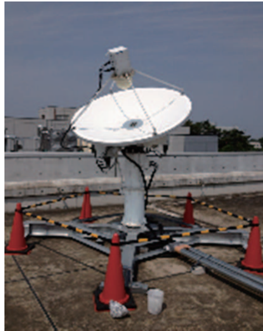
Fig. 1 MARBLE1 compact station on the roof of NMIJ building in Tsukuba
