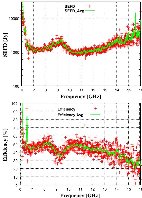
**Fig. 4** SEFD(upper) and aperture efficiency(lower) of 34m antenna with IGUANA-H feed.
