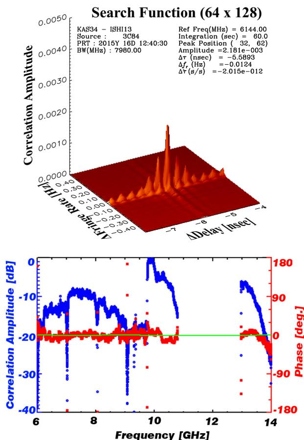
Fig. 7 A fringe obtained by 8GHz bandwidth synthesis (upper panel) and phase and Amplitude of the cross spectrum (lower panel). Amplitude variation over the frequency is caused by differences of data acquisition systems and signal paths. Inter-band and Intra-band phase characteristic correction has been applied.
