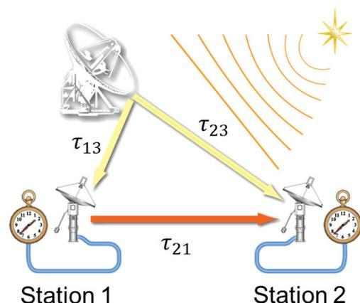
Fig. 1 Concept of GALA-V project for distant frequency comparison.
