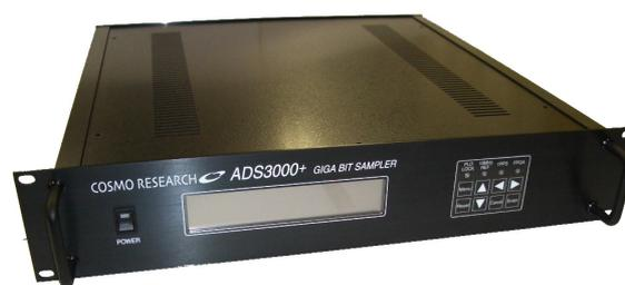
**Fig. 5** Outlook of ADS3000+. One set of sampler is capable of “64Msps x 2bit x 16ch” observation.
