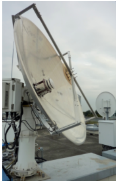
Fig. 2 Renewed MARBLE with 2.4m dish and the NINJA feed
